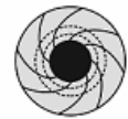
Relative position of the iris diaphragm of the objective and the image of a ring diaphragm of the condenser in the exit pupil of the objective during central screening
