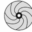
Relative position of the iris diaphragm of the objective and the image of a "point" diaphragm of the condenser in the exit pupil of the objective during ring screening
